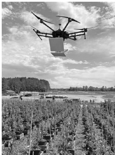
Clemson University researchers test a drone that can be used to scan radio frequency identification tags on pots in plant nurseries for quick, accurate inventory. Currently, researchers are evaluating the best tag placement and drone flight plans. Photo by Joe Mari Maja, Clemson University.
