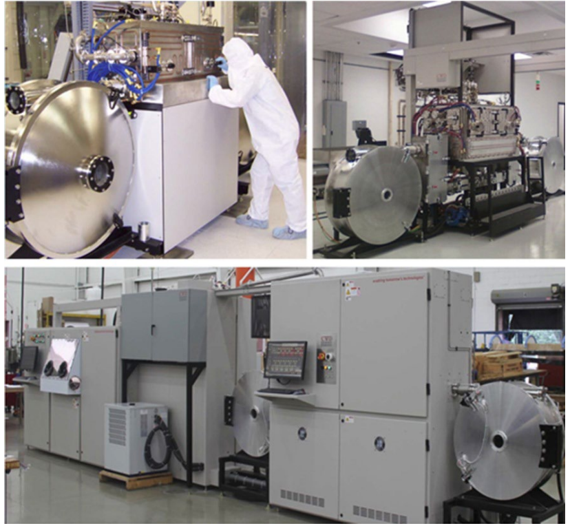
Advanced “Roll-to-Roll” Manufacturing Technologies developed at the joint UH-Superpower, Inc. facility located UH-ERP enabling industrial scale production of 2G high temperature superconducting materials
